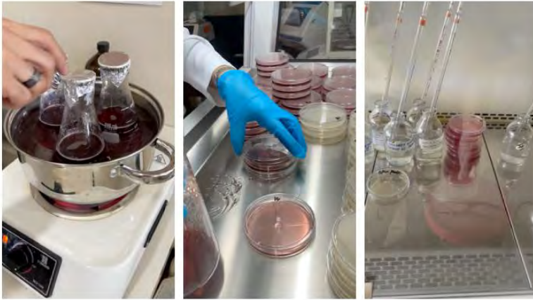
Figure 3. Determination of Fecal Coliforms and Total Coliforms (r-l: Preparation of VRBA, Pour plating, Interpretation)
