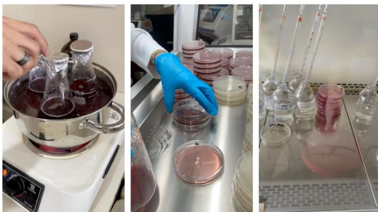
Figure 3. Determination of Fecal Coliforms and Total Coliforms (r-l: Preparation of VRBA, Pour plating, Interpretation)
