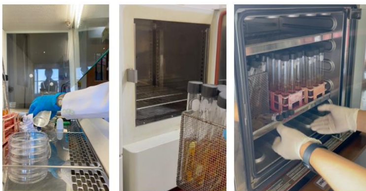
Figure 1. Determination of Total Coliforms (r-l: MTT, Incubation, Interpretation)
